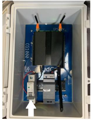
3. Within a few minutes of receiving power the status LEDs (next to the GPS antenna) should all turn green.
