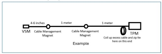
6. We DO NOT recommend adjusting the length of the integral cable between the VSM and TPM as this will void your warranty. Our recommendation is to coil up any excess cable **near the TPM side of the installation** using the heavy duty, UV-resistive zip ties provided by Machine Saver. You are also welcome to purchase AirVibes with custom cable lengths, for more information on custom integral cable lengths, please reach out to sales@machinesaver.net or call +1(832)581-9908 for more information.
