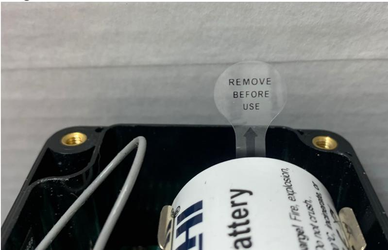
3. After removing the Tab the Buzzer might make some noise.
