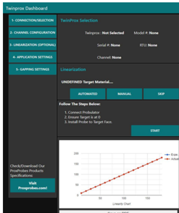
Figure 5: The TwinProx software features a simple, intuitive user interface that makes it easy to configure TwinProx in the field.
